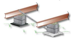
130-172 5' Xi 2 Ground System with Lateral Strut & Hardware
